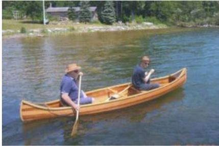
The shell of the canoe is made of cedar strips 3/4" wide and 1/4" thick. Each strip has to be shaped to fit and the entire hull is then sealed with a fibreglass coating and varnished numerous times.
